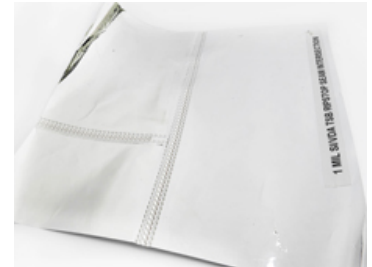
Close up of the Kapton material that the Webb Sunshield was created from. Credit: NASA
