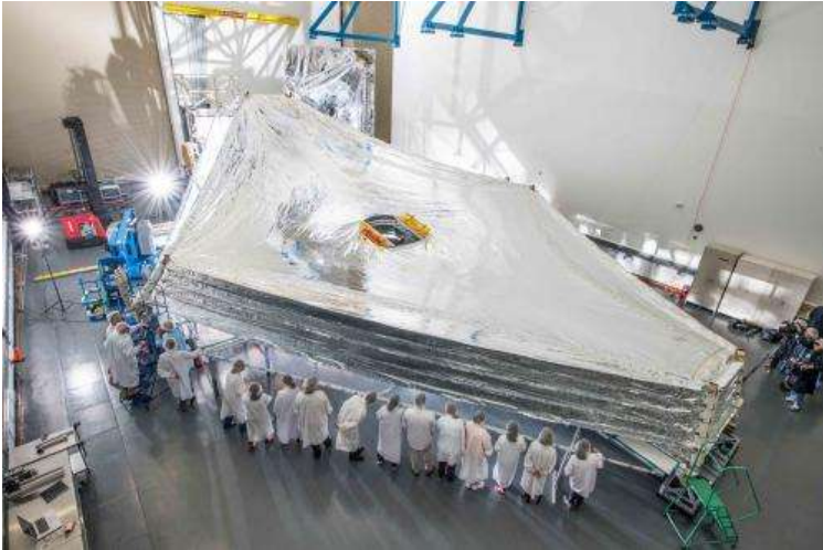
The sunshield test unit on NASA's James Webb Space Telescope is unfurled for the first time. Credit: NASA
