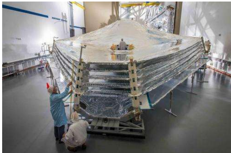
Sunshield test unit on NASA's James Webb Space Telescope is unfurled for the first time at Northrup Grumman. Credit: NASA
