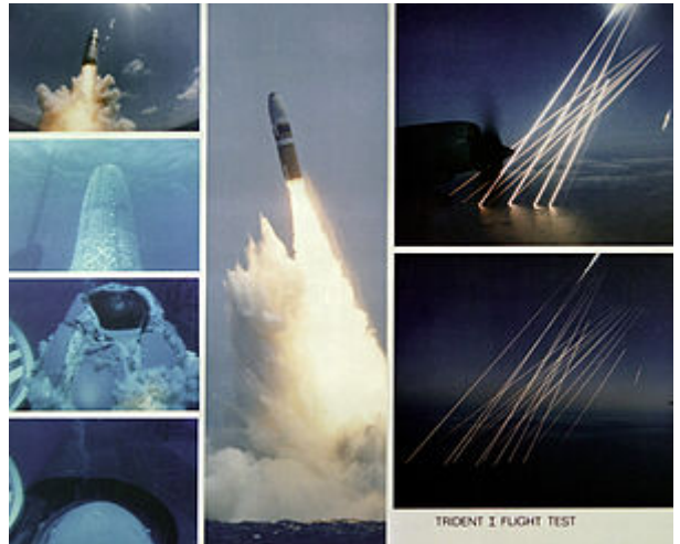
The launching of a Trident I C-4 missile from the submerged USS Francis Scott Key and the re-entry vehicles plunging into the Atlantic Ocean, 1981
