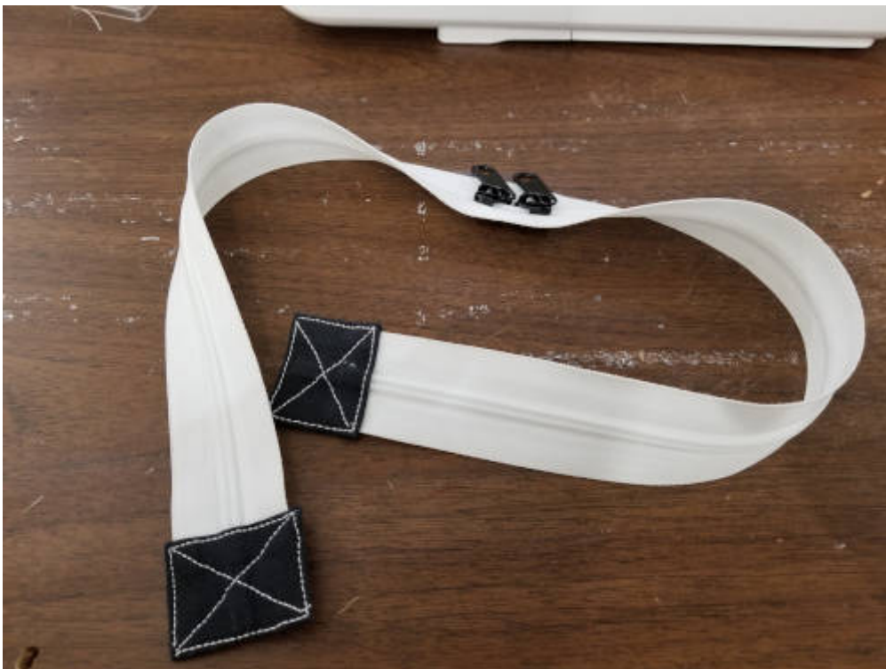
Zipper ends attached to the zipper
