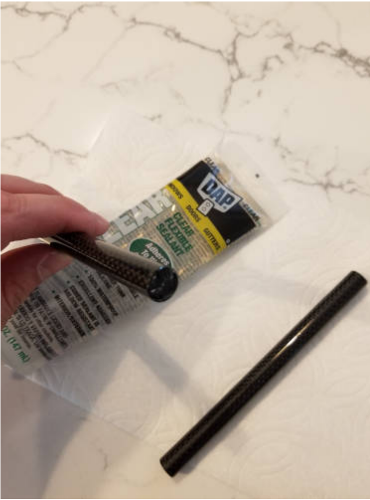
Filling the end of the tube with sealant
