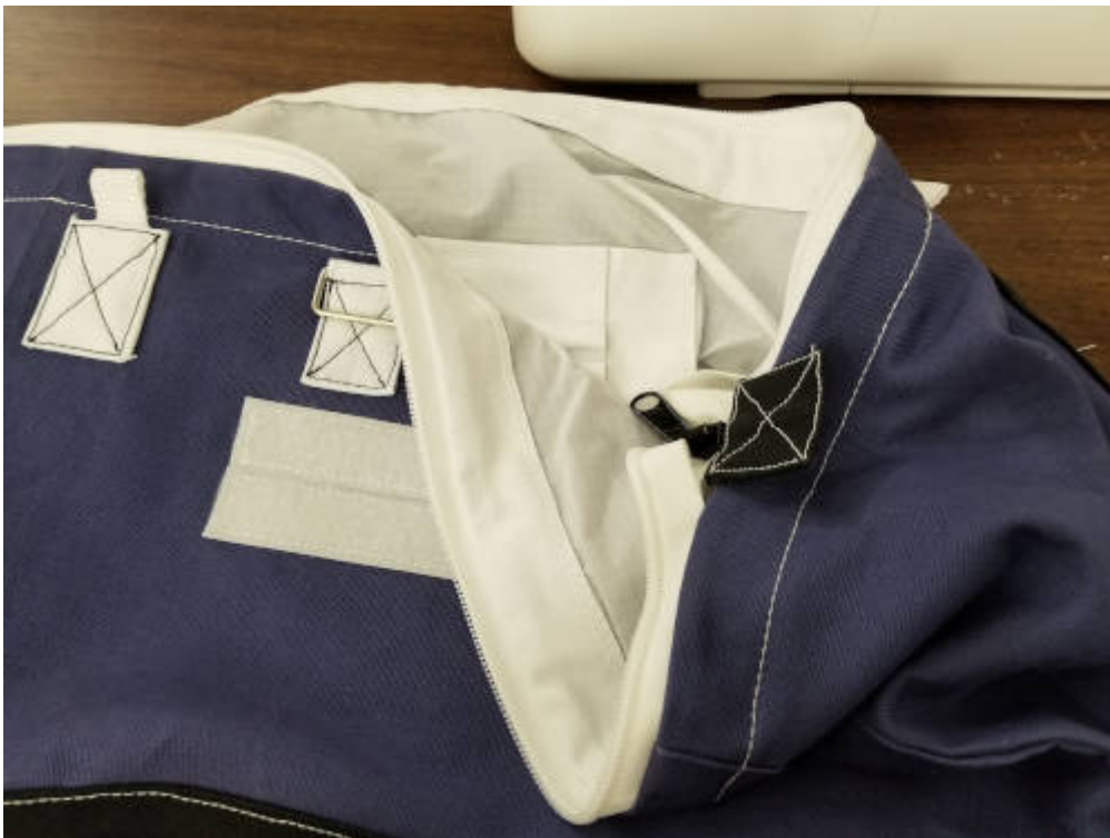
Frame channel sewn down
