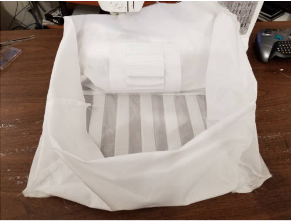
Lining bottom attached to sides
