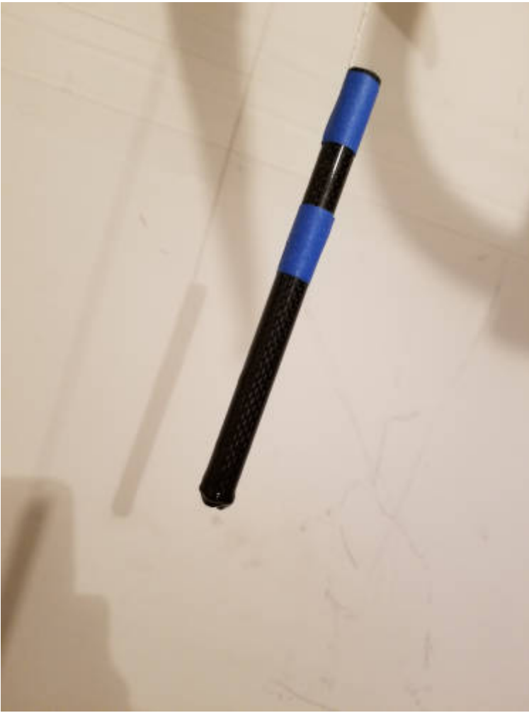
Drying the Plasti-Dip on the handle tube
