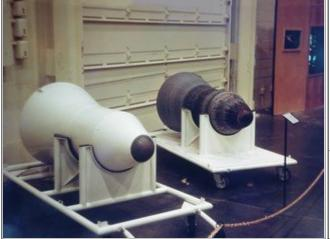
Minuteman missile nose cones. A intact nose cone at left, one that was used for a re-entry test at right. The outer casing is meant to wear off, or ablate, to shed reentry heat.
