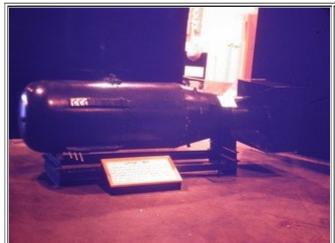
"Little Boy" was the atomic bomb dropped on Hiroshima. It was a "gun type" weapon, meaning two pieces of uranium were fired together at high speed to form a critical mass. This configuration was considered such a sure thing there was no felt need for a test.
