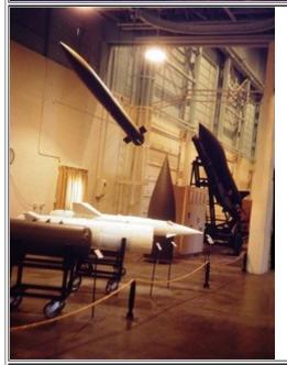
A variety of weapon configurations in the foreground. The hanging rocket is an artillery rocket called Little John. The rocket in the background with the bulbous nose is the Honest John, which was first deployed in 1953 and finally retired in 1982. The large upright nose cone is from a Corporal missile.
