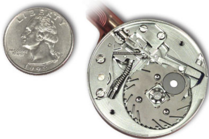
A mechanical safe arming detonator (MSAD) prevents accidental or unintended detonation of a nuclear warhead. Stockpile stewards at Livermore are working on an advanced MSAD for the W78.
