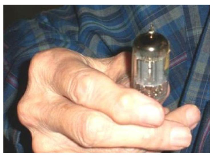
Bob Peurifoy holding the 12AU7 vacuum tube. Bob notes: "It was manufactured by Sylvania Electric in August 1959. It still meets new tube specifications. It is representative of the types of vacuum tubes used in the B61 vacuum tube radar."
